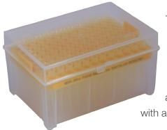
The practical and reusable pipette tip holder with the CE & IVD certified pipette tips are already inserted and make everyday laboratory work easier. The holders are neatly stored in a box that can be autoclaved up to ten times. The pipette tips can be securely attached to the Elegant Pipette or other commercially available micropipettes. They seal tightly and are absolutely leak-proof. In addition, the pipette tips are equipped
