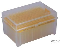
The practical and reusable pipette tip holder with the CE & IVD certified pipette tips are already inserted and make everyday laboratory work easier. The holders are neatly stored in a box that can be autoclaved up to ten times. The pipette tips can be securely attached to the Elegant Pipette or other commercially available micropipettes. They seal tightly and are absolutely leak-proof. In addition, the pipette tips are equipped with a special filter that prevents contamination.
